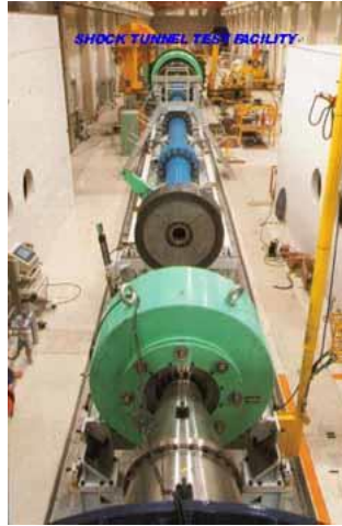
Figure 16: Shock-wind tunnel at Mitsubishi Heavy Industries.
