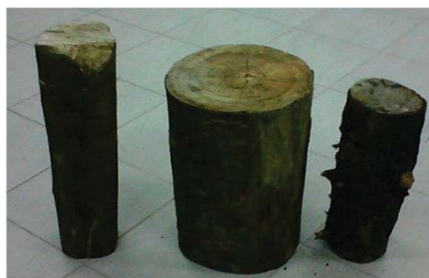
Fig. 5. The three species of wood studied (caixeta, garapuvu, and pine, from left to right).
