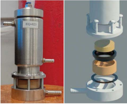
Fig. 7. Filter pilot for the dead-end filtration.
