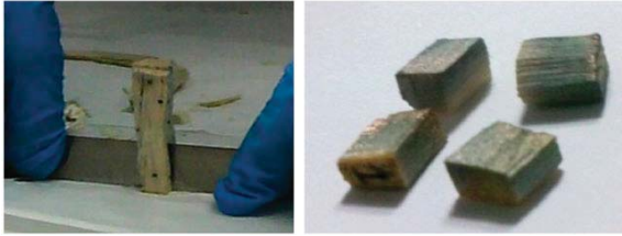
Fig. 11. Samples of wood during the cutting process and prepared with the gold covering.
