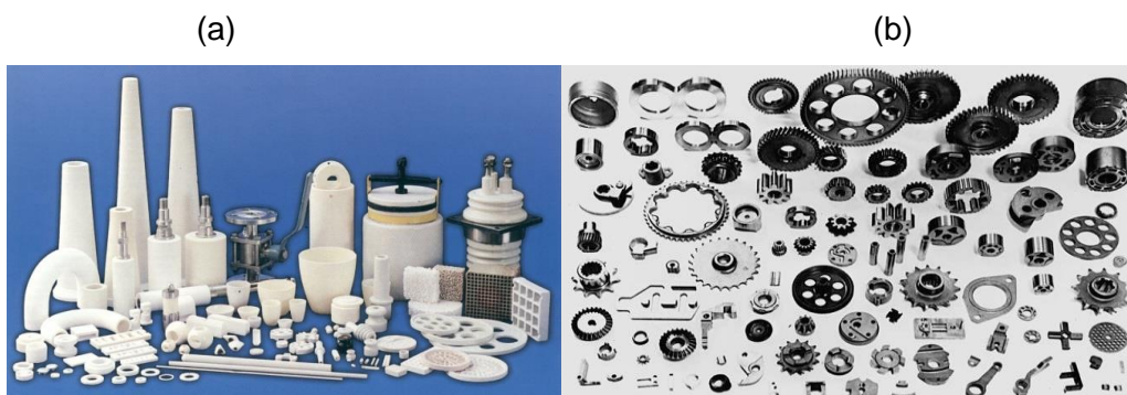
Figure 1 - (a) examples of advanced ceramic applications and (b) examples of powder metallurgy products.
