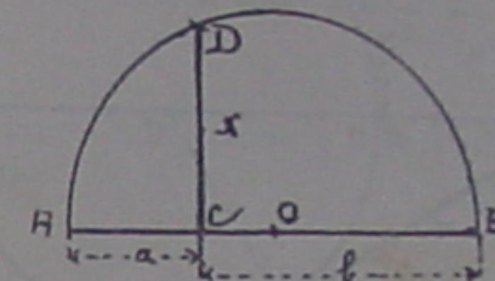
$$\begin{aligned}\frac{a}{x} &= \frac{x}{b} \\ x^2 &= ab \\ x &= \sqrt{ab}\end{aligned}$$
