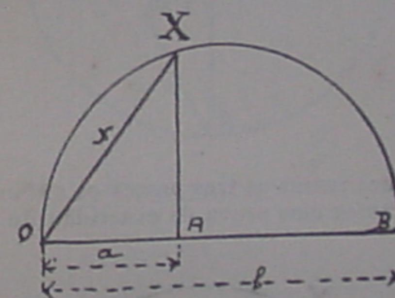
$$\begin{aligned}\frac{OA}{OX} &= \frac{OX}{OB} \quad \frac{a}{x} = \frac{x}{b} \\ x^2 &= ab \\ x &= \sqrt{ab}\end{aligned}$$
