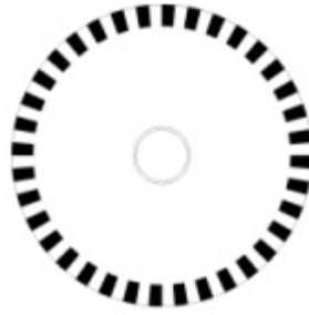
Figure 29 - Incremental encoder disk. [ 13 ]
