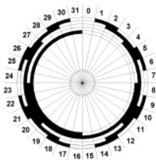
Figure 30 - Absolute encoder disk. [ 13 ]
