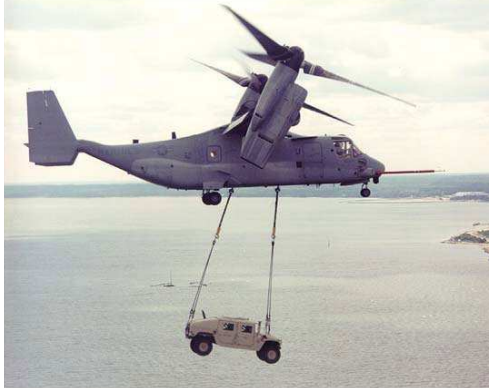
Figure 1 – Bell-Boeing V-22 Osprey in cargo transportation task
