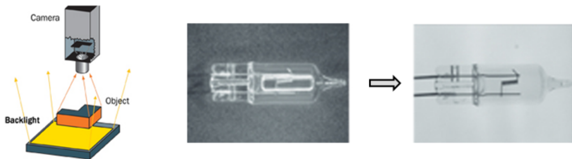
Figure 3.10: Light bulb: Resulting image clearly shows silhouette of filament inside the bulb [9].
