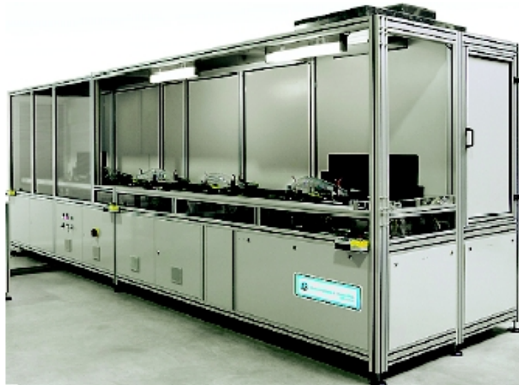
Figure 1.1: Industrial machine for the automated inspection of free formed surfaces.
