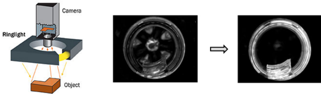
Figure 3.9: Plastic bottle: Defect on top of a plastic bottle is clearly identified.[9].
