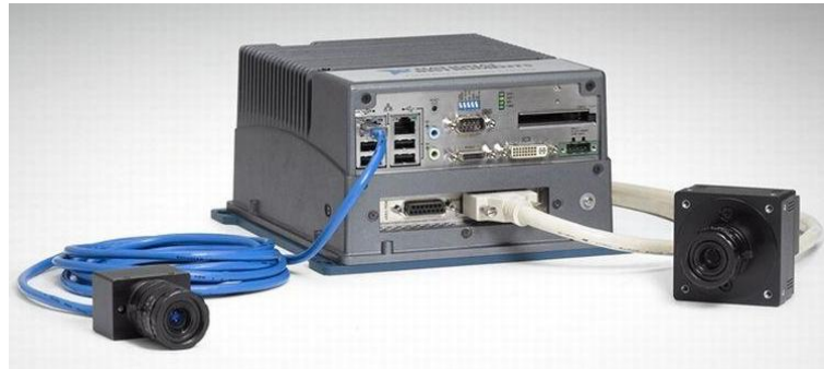
Figure 3.6: National Instruments EVS.
