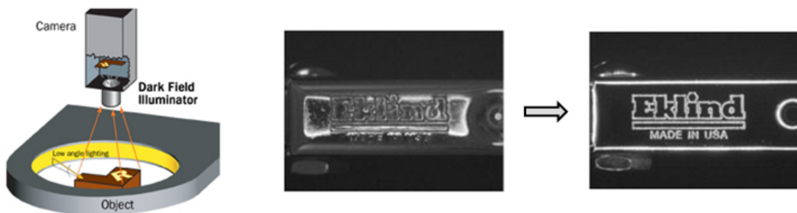
Figure 3.8: Embossed logo on a metal surface: Low angle illumination provides a high contrast [9].
