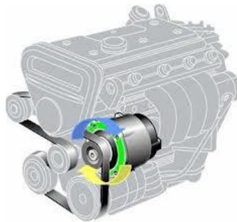
Figure 1: Generator being activated by the engine belt 1 .
