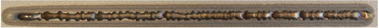
Figure 6-2: Surface of the track cladded with maximum traverse speed and minimum laser power. The energy per length unit is not high enough to melt the wire properly.
