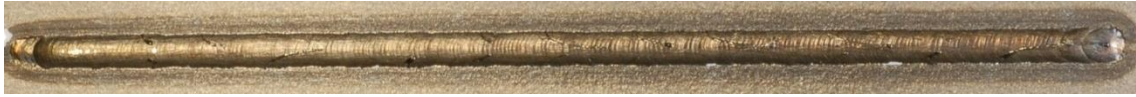
Figure 5-9: Track surface cladded with 770 W, at 5.83 mm/s. There is a region without wire on the beginning (left), created because the wire was placed too far away from the substrate.
