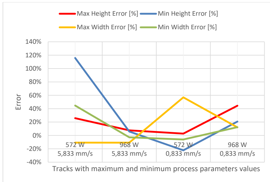
Figure 6-8: Prediction errors of track dimensions. The horizontal axis represents the different tracks clad with the maximum and minimum process parameters values. Tracks are ordered by energy per length rate level.
