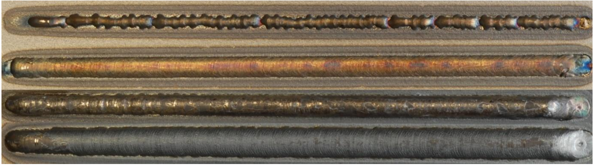
Figure 6-3: Tracks clad with the maximum and minimum parameters values. Tracks are sorted by energy per length unit rate, from lowest (top track) to highest (bottom track).
