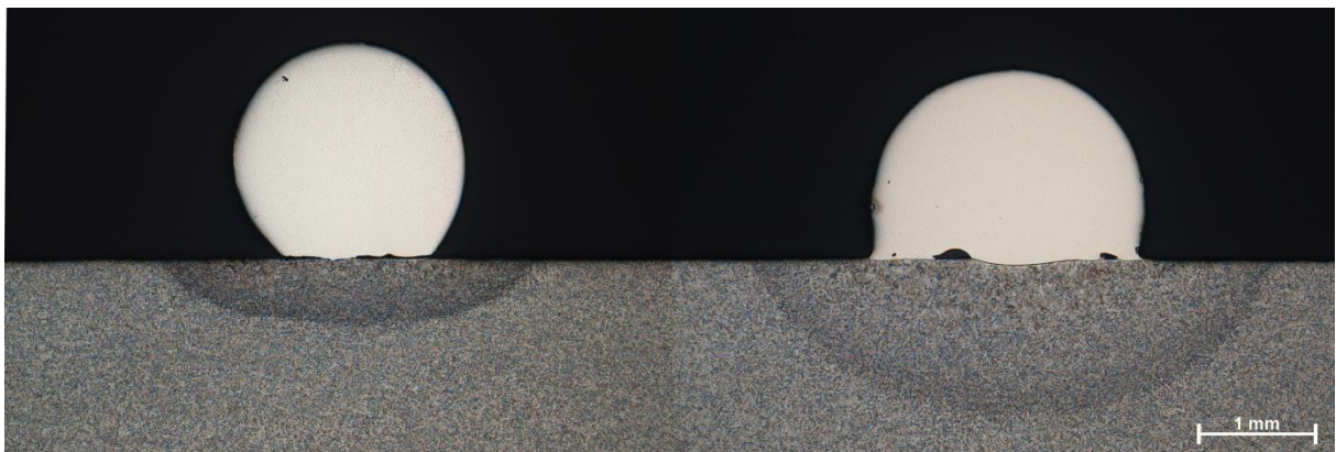
Figure 6-9: Cross sections of the beginning (left) and of the end (right) of the track with the minimum process parameters values. Molten pool width is larger on this track's end.
