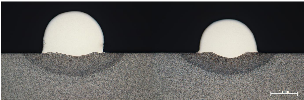
Figure 5-10: First cross sections of the track obtained at 0.83 mm/s (left) and at 1.15 mm/s (right). Volume of the track at the left is the biggest, explaining this shielding effect.
