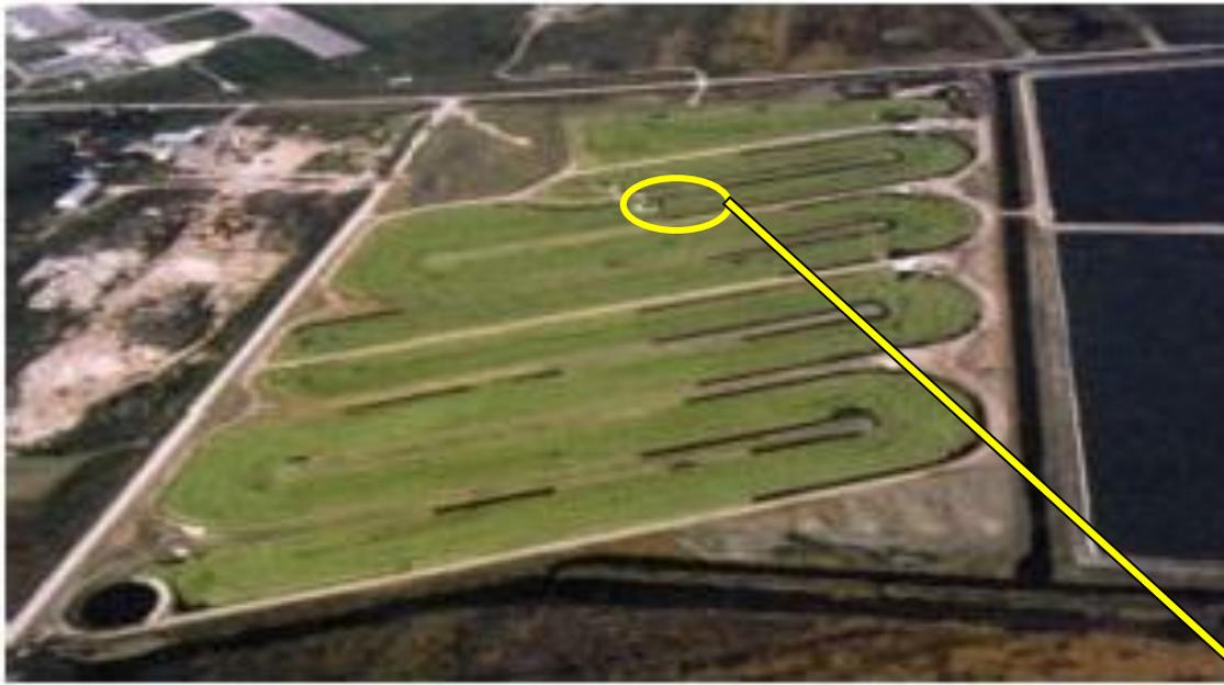
*Photograph 2: Duckweed-covered serpentine plug-flow lagoon in the USA for tertiary treatment of effluent from three facultative lagoons followed by a wetland buffer. Design flow is reported at 19,000 m<sup>3</sup>/d, with peak flows reaching 38,000 m<sup>3</sup>/d. (Photograph: Lemna Corp. 1994).*
