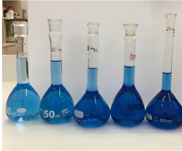
Figure 7 – Dye solutions in concentrations of 5, 10, 15, 20 and 25 mg/L from the left to the right.
