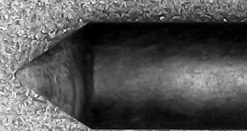
A black and white photograph of the same electrode tip after welding. The tip is significantly wider and has a more rounded, irregular shape. A 1 mm scale bar is located at the bottom left of the image.<br>1 mm |
