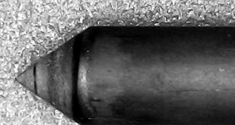
A black and white photograph of the same electrode tip after welding. The tip is wider and has a more rounded, irregular shape. A 1 mm scale bar is located at the bottom left of the image.<br>1 mm               |
