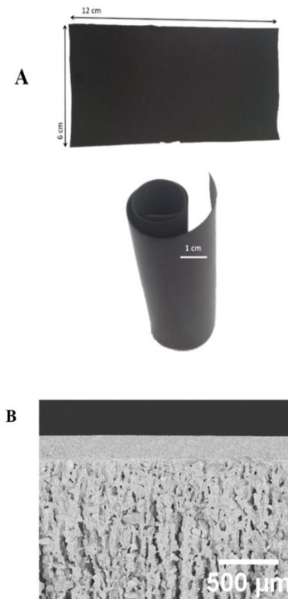
Figure 34. (A) General view of a green tape of LSCF. (B) Sintered tape and support.
