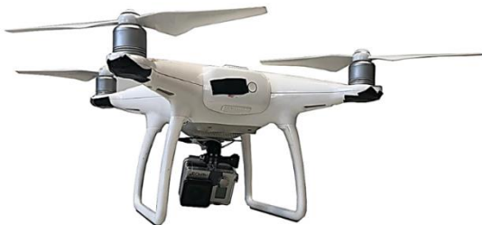
Figura 20 – GoPro HERO 3 Plus Black® adaptada a um Drone DJI Phantom 4 Pro
