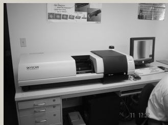
Figure 1 – Skyscan 1072 μ-CT system used to study the sandstone samples. The equipment is simple to operate and the resolution depends on sample size and composition. PETROBRÁS Research and Development Center (CENPES), Rio de Janeiro, RJ, Brazil.
