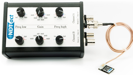
Figure 7 – champs 1.1 - iNDTact Amplifier. It was used during the tests to filter the signal measured from the AE sensor.
