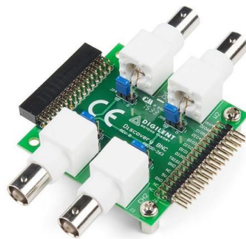
Figure 17 – BNC board. It is an external device that goes attached to the Analog Discovery 2. Allow connecting BNC cables (oscilloscope standard cables) to the Analog Discovery 2.
