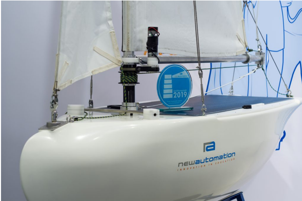
Figure 1 – Prototype II developed by the STDA, comprised of a 2.20m long fuselage, mainsail, jib, expanded sensor system, and a completely self-sufficient energy supply provided by a solar panel (Image included with permission from Sailing Team Darmstadt e.V.)
