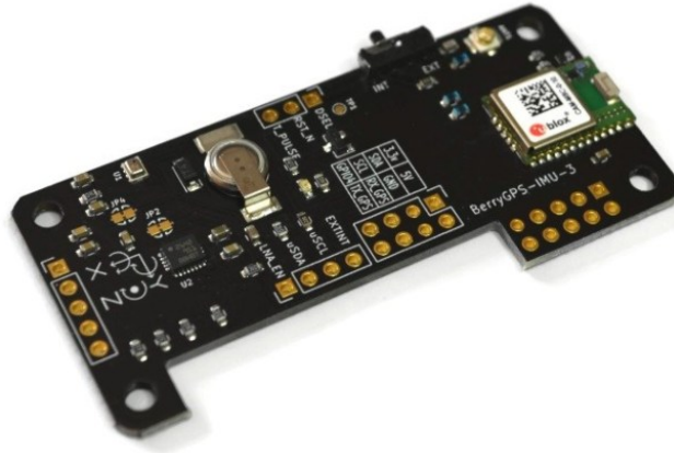
Figure 6 – Module BerryGPS-IMU, which provided the values for the measurement noises to generate more realistic simulations. It contains a GPS module, to the right and a IMU to the left
