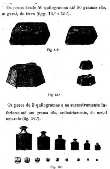
Fig. 9. Pictures of iron weights to measure weight between 50kg and 50gr (left) and weights of less than 1gr – made by yellow metal – (right). (Carvalho, 1912, pp. 103-104)
