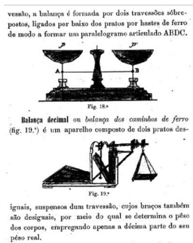
Fig. 10. Balances' illustrations after its description. Decimal balance with other name: railway scale (it was used at train stations to measure luggage and packages weight) (Carvalho, 1912, p. 106)
