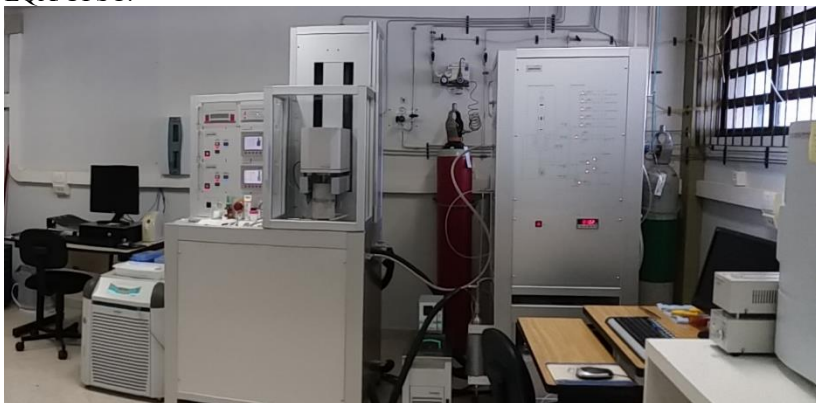
Figura 7 - Termobalança Dyntherm HP-ST (Rubotherm) instalada no LEMA/ EQA/UFSC.
