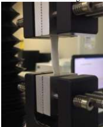
Figure 8 - Samples fixation for tensile strength test.
