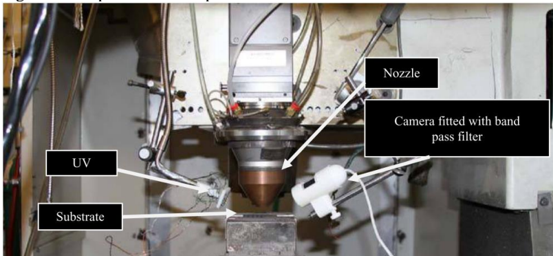
Figure 10- Experimental setup with a webcam and UV illumination.
