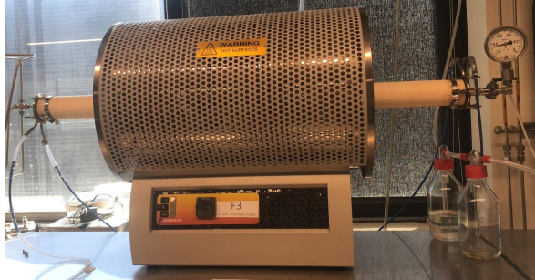
Figure 54: Furnace for preceramic precursor, dense and porous pieces pyrolysis using argon as atmosphere up to 1100 °C.
