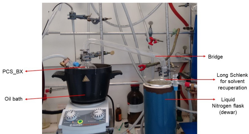
Figure 38: Scheme for toluene (solvent) removal from hydroboration synthesis.
