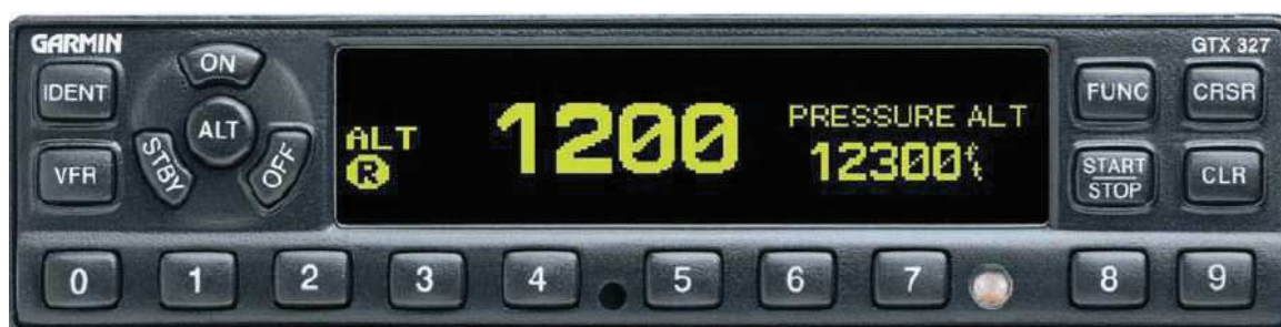
Figura 19 – Painel de controle do Transponder
