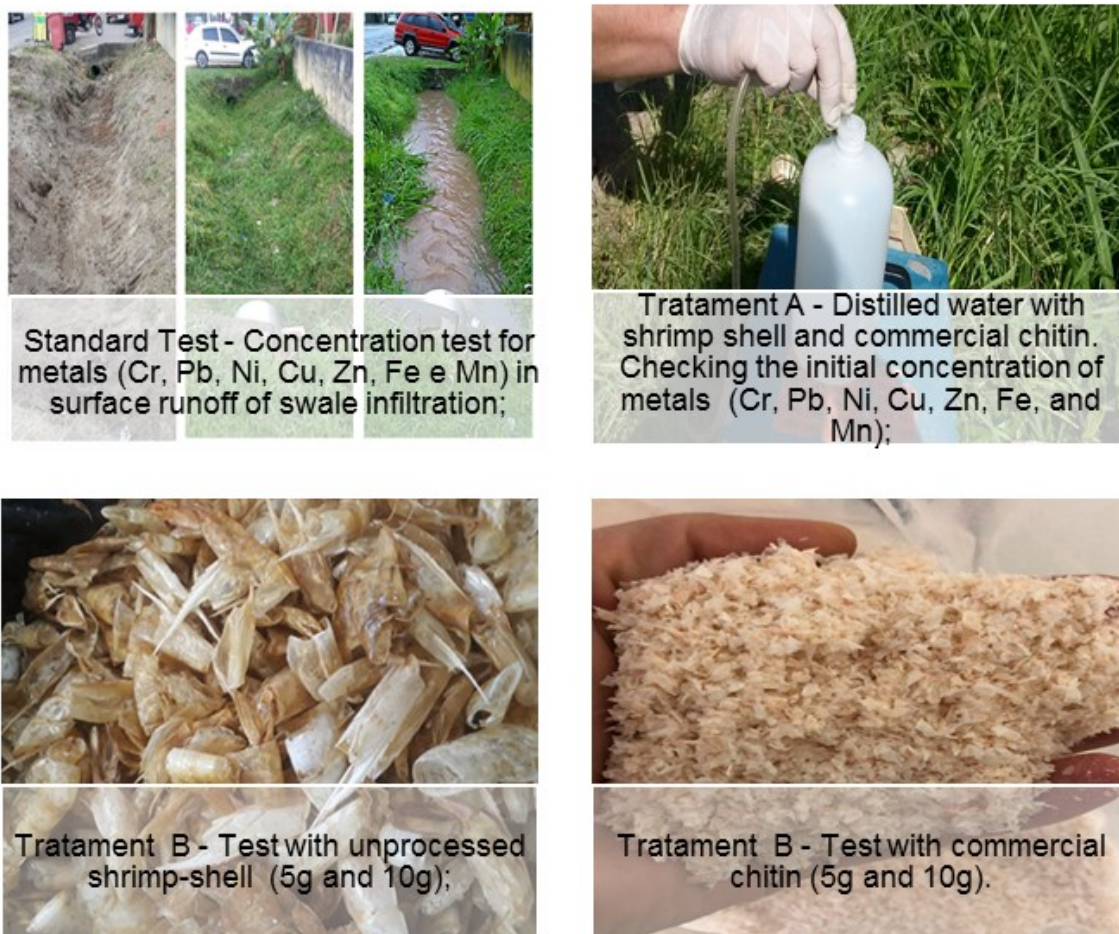
Figure 5-2. Procedures used in this research: surface runoff pattern; white test in biosorbents and treatments with shrimp shell and commercial chitin.
