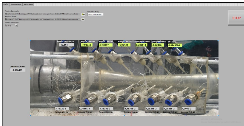
Figure 21 - Photograph of the software main screen with pressure drop measurements along the Venturi.
