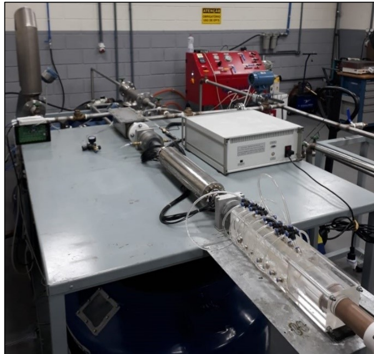
Figure 15 - Photograph of the multiphase flow experimental setup.
