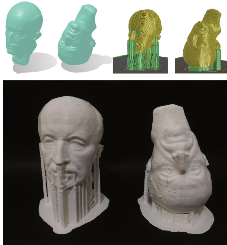
Figure 3.1.8: Surface decimated-max.obj on the initial vertex position (top-left) and after rotation (top-center-left). The same surface on the initial position on the printing simulator (top-center-right) and after rotation (top-right). In yellow, the software indicates the solid that we want to print and in green the overhang supports. The bottom figure is a photo of the same surface after printed. On the bottom-left, the surface is at the initial vertex positions and on the bottom-right, the surface is positioned after rotation.
