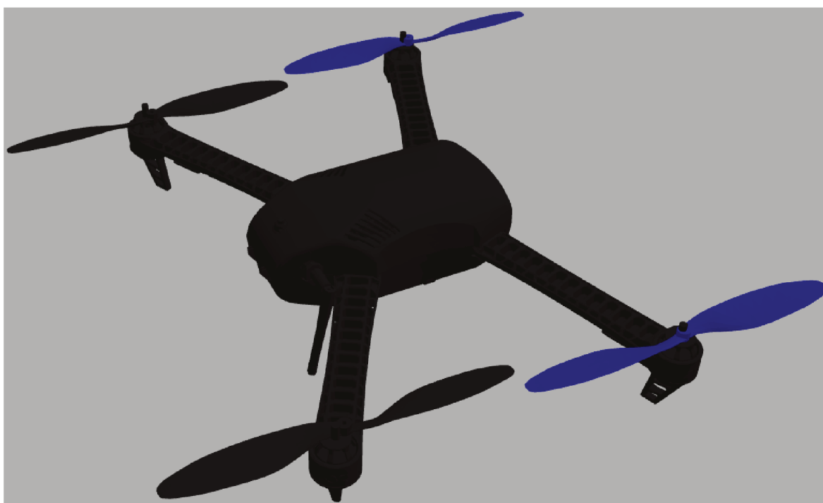
Figure 1 – Screenshot of the Iris drone model, the blue blades indicate the front of the drone. Conventional drone.
