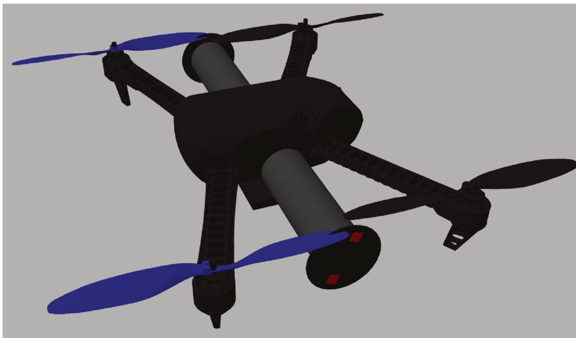
Figure 2 – Iris model with the Magnus wings model attached to it, composing the Hybrid Drone model.
