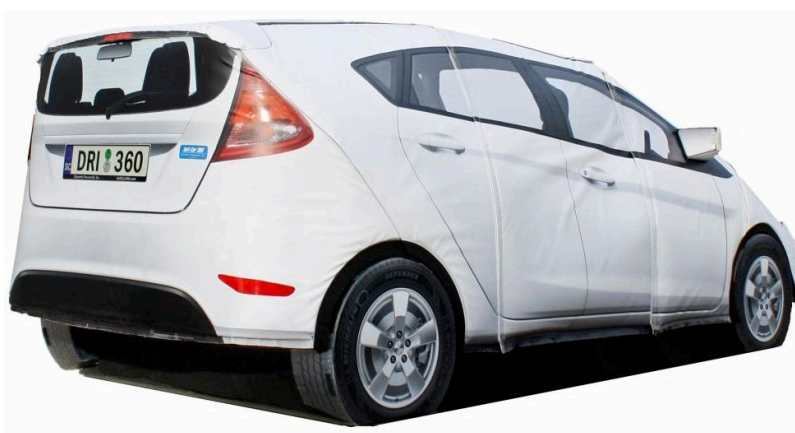
Figure 10 – The global vehicle target (GVT).
