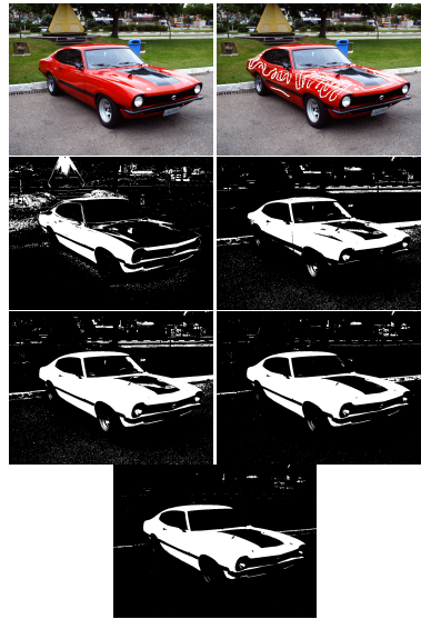
Figure 2. Thresholded images based on the value of the distance between each pixel of the first image and a reference pixel, marked in the second image on the right side of the car.
