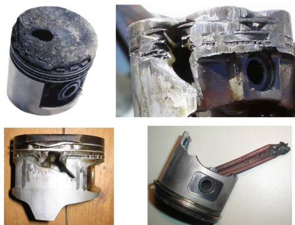
Figure 2. Damages in internal combustion engines caused by operating on knocking regime
