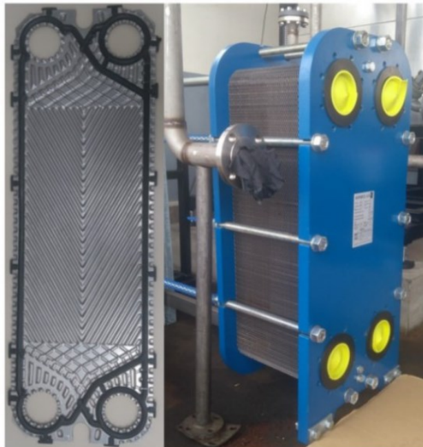
Figure 1 – Gasketed Plate Heat Exchanger. Left: front view of a plate with the gasket. Right: a mounted gasketed plate heat exchanger.
