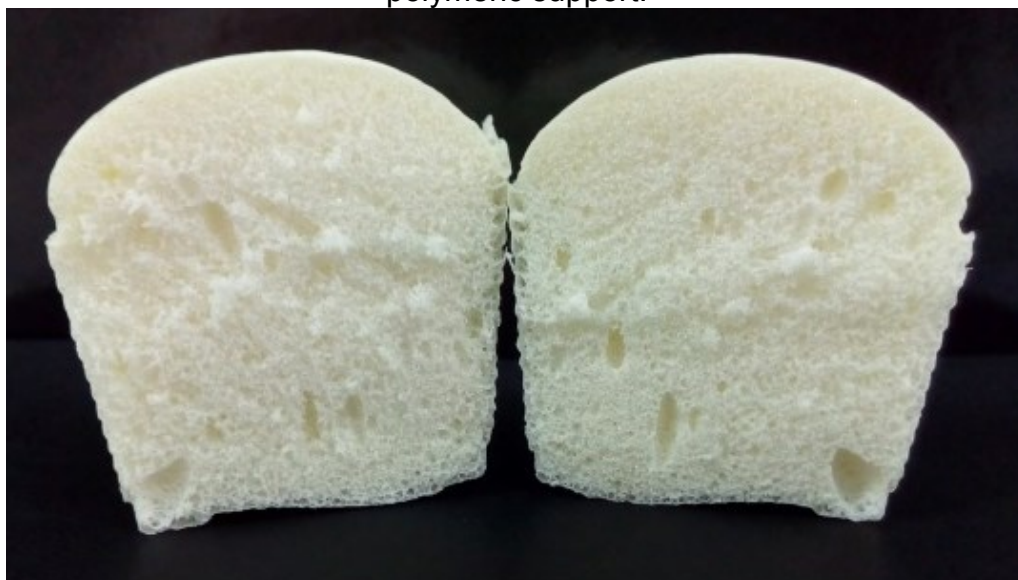
Figure 12 - Soluble Eversa® Transform 2.0 lipase immobilized on polyurethane polymeric support.
