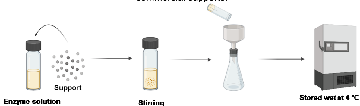
Figure 25 - Scheme of soluble Eversa® Transform 2.0 lipase immobilization in commercial supports.
