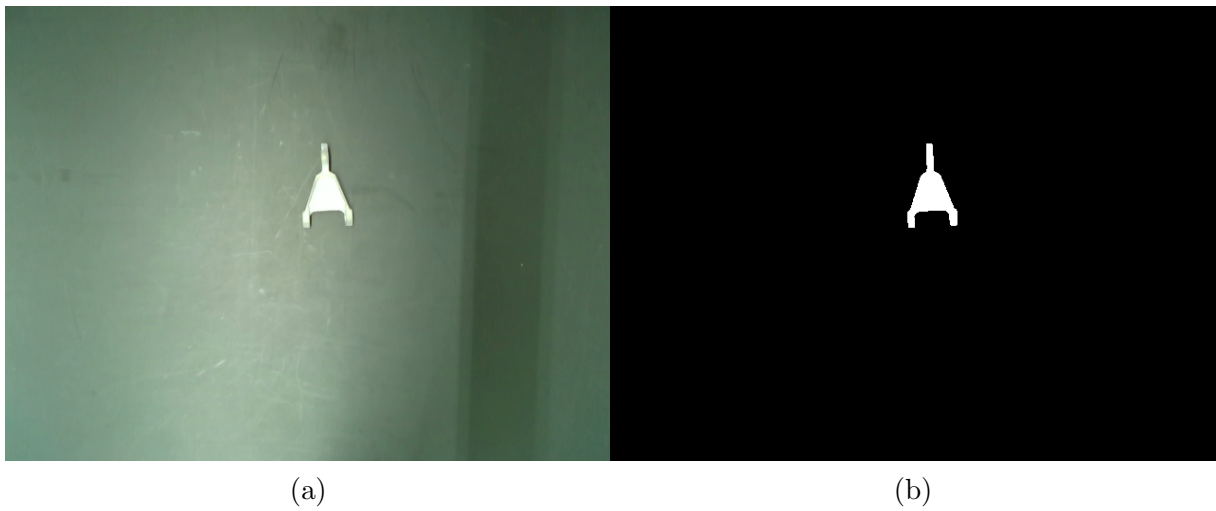
Figure 22: Comparison between (a) RGB image without filtering and its (b) segmentation applied to the aircraft part.
