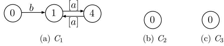
Figure 28 – Cluster automata C_1 , C_2 , and C_3 after observation of event b .
