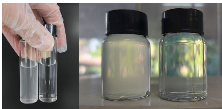
Figure 5.11 Visual comparison between oily wastewater feed (250 ppm) and permeate.
