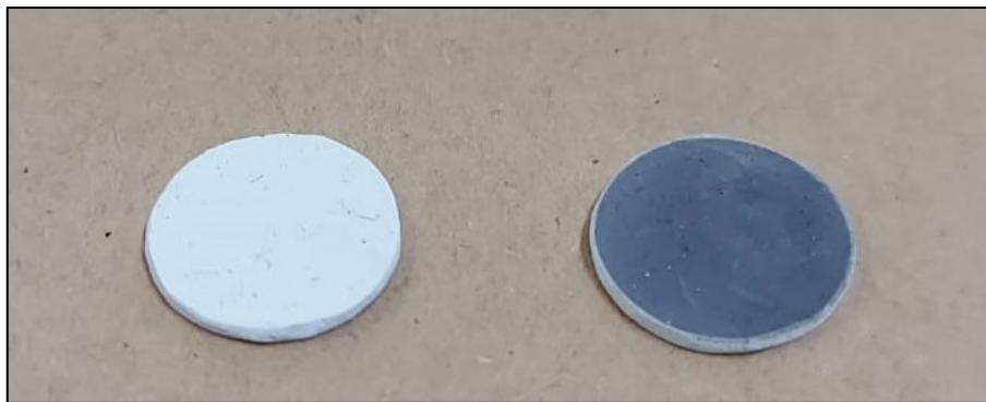
Figure 5.9. PM membranes after filtration of acetaminophen, in dark conditions (white) and under UV (gray).
