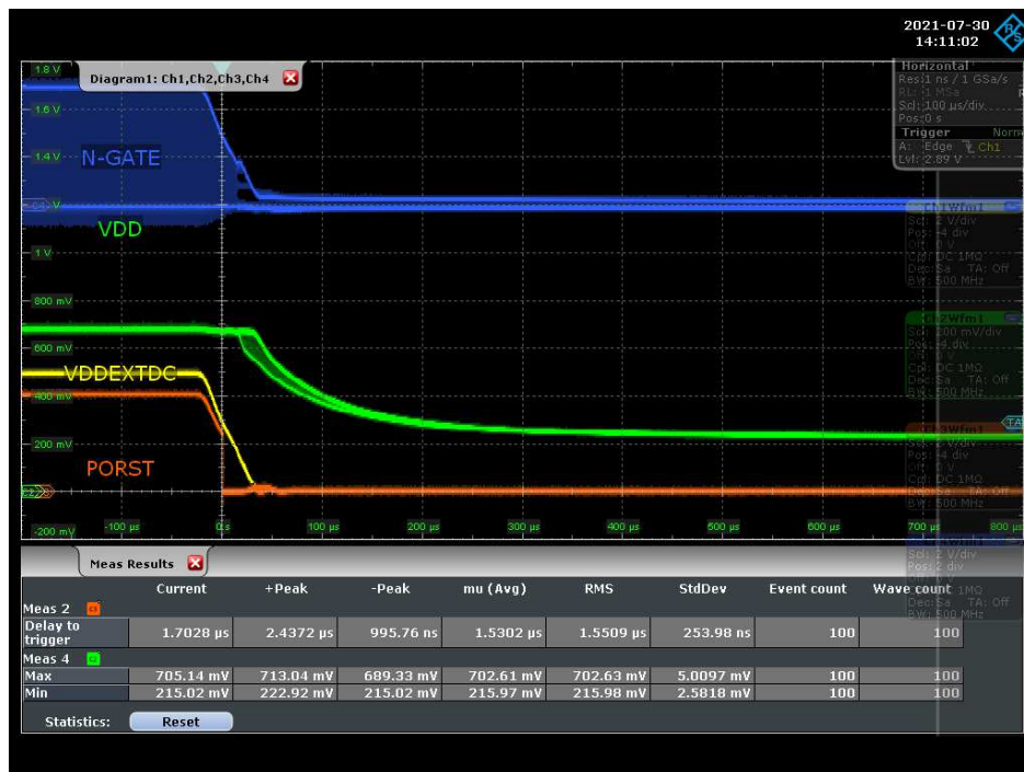
Figure 29 - EVRC Supply Fail
