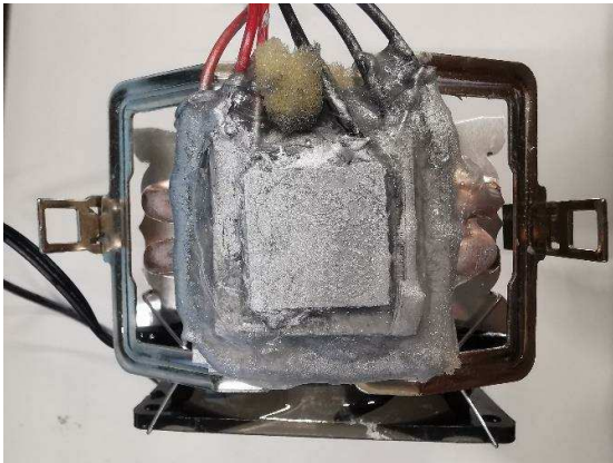
Figure 35 - Peltier modules fixed on heatsink
