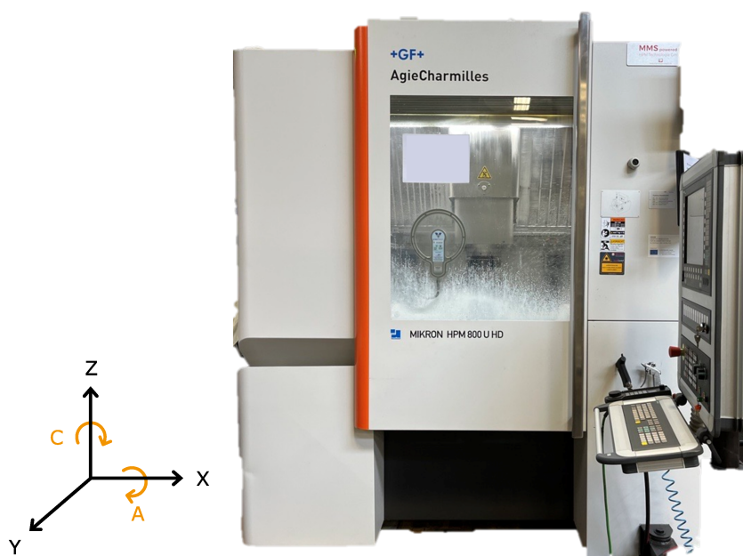
Figure 15 – Mikron Vertical Machining Center with Five Axis
