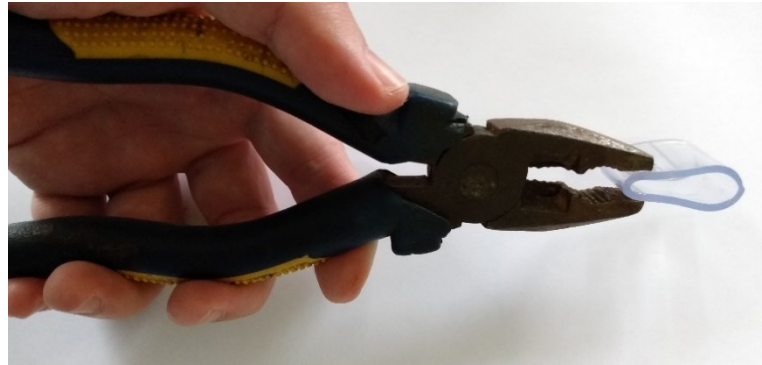
Figure 63 - Reshaping the chamber to an elliptical format.
