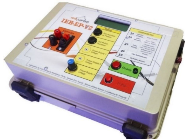
Figure 11 – PEF equipment prototypes: (a) up to 120 V, 10 A, monopolar, with fine voltage adjustment; (b) up to 800 V, 20 A, monopolar, with embedded current-voltage datalogger; (c) up to 800 V, 30 A, bipolar, with embedded current-voltage datalogger and its electronics (d). (e) European Standard Operating Procedures of Electrochemotherapy (ESOPE) adapted pulse (800V, 20 A, 100 \mu s monopolar, 5 kHz repetition rate eight pulse train).
