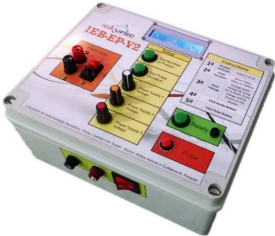
Figure 11 – PEF equipment prototypes: (a) up to 120 V, 10 A, monopolar, with fine voltage adjustment; (b) up to 800 V, 20 A, monopolar, with embedded current-voltage datalogger; (c) up to 800 V, 30 A, bipolar, with embedded current-voltage datalogger and its electronics (d). (e) European Standard Operating Procedures of Electrochemotherapy (ESOPE) adapted pulse (800V, 20 A, 100 \mu s monopolar, 5 kHz repetition rate eight pulse train).
