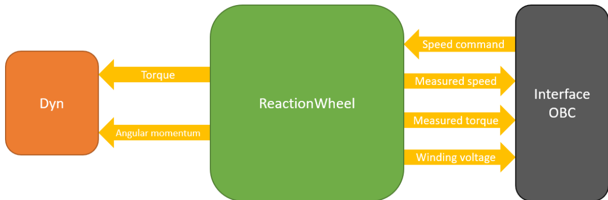
Figure 32 – The interfaces of the reaction wheel model.
