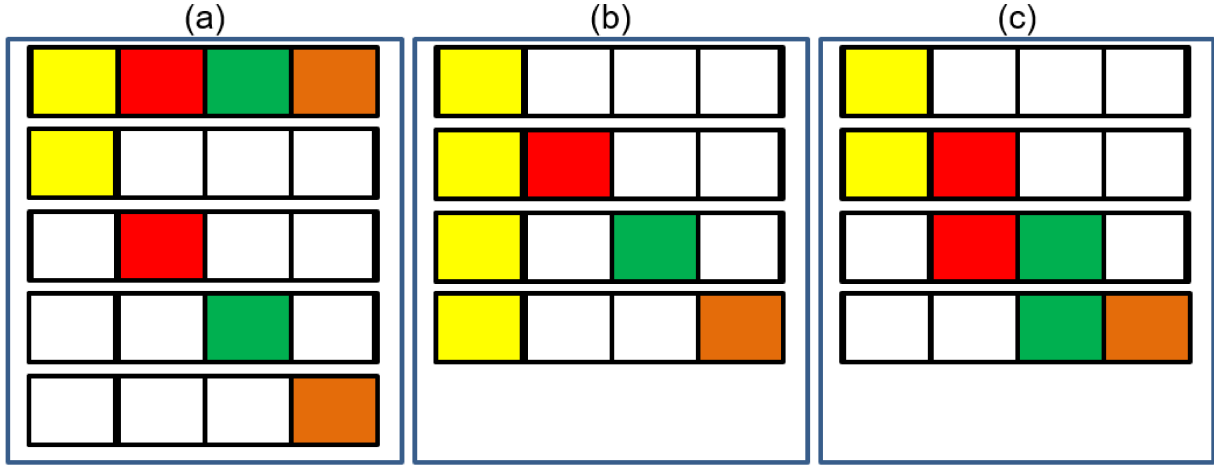
Figure 18 – Schematic of optimization problems with a particular structure, where (a) contain complicating constraints, (b) complicating variables, and (c) is partially coupled.
