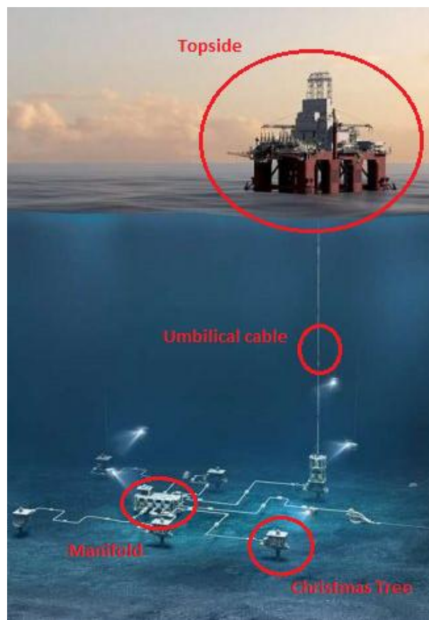
Figure 21 – Subsea production system.
