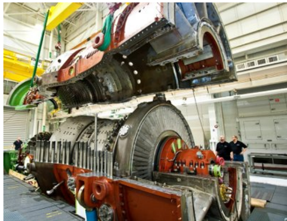
Figure 2 – Gas turbine with housing
