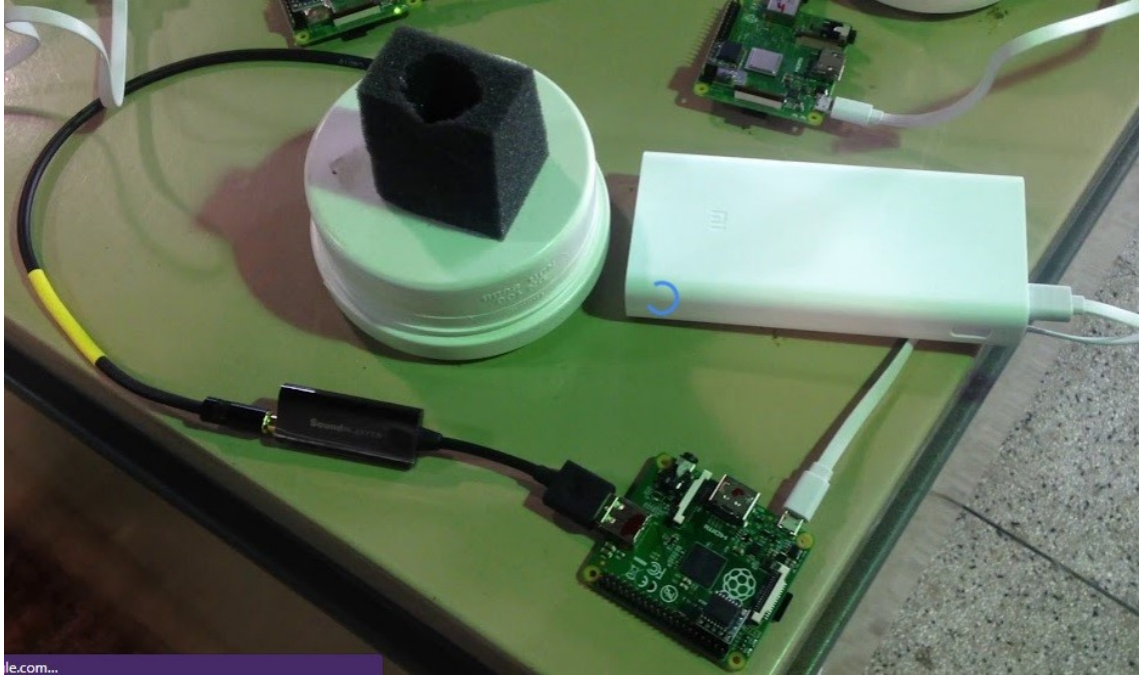
Figure 2: The SOLO audio recorder: a Raspberry Pi A+ board connected to a power bank and a hydrophone (attached to the PVC cap).
