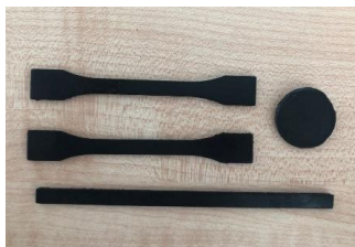
Figure 3-3: Compression molded samples used for different tests.
