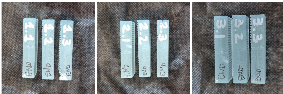
Figure 22 – Glass test-pieces used for removal rate investigations. Each one with its own identifier.
