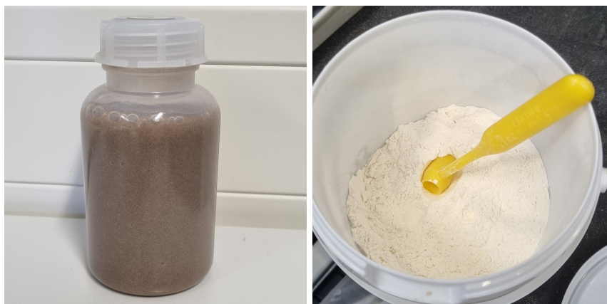
Figure 11 – Example of slurry mixture (on the left), containing the thickener (showed on the right).
