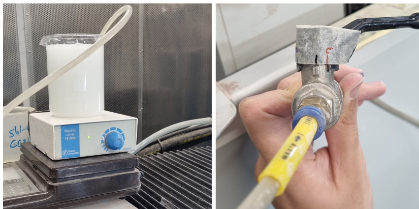
Figure 10 – Parts necessary to set up slurry injection in the AWJ system.
