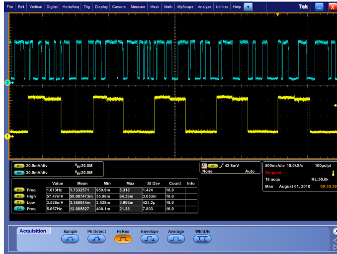
Figure 34 – Output signals of both frequency divider chains at 76 mV of supply voltage
