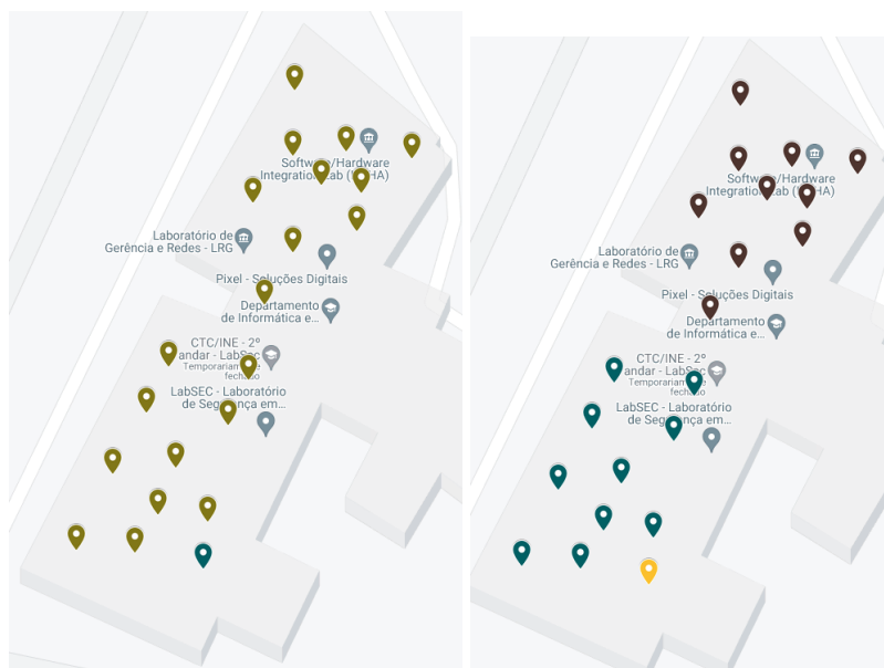
Figure 32 – 20 nodes with 1 region on the left and 2 on the right in the INE E2 scenario
