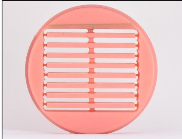
**Figure 1-** PMMA block (Ivotion® Base Pink-V, Ivoclar Vivadent® AG, Liechtenstein) milled to the dimensions established in the design software.
