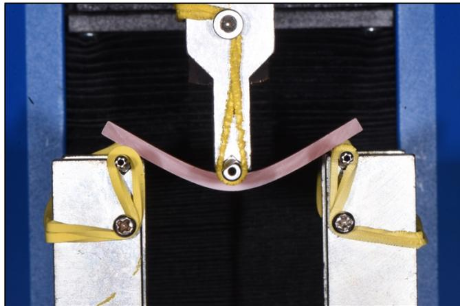
**Figure 4-** Specimen being subjected to the 3-point flexural strength test on a universal testing machine (Instron<sup>®</sup> EMIC 23-5S).
