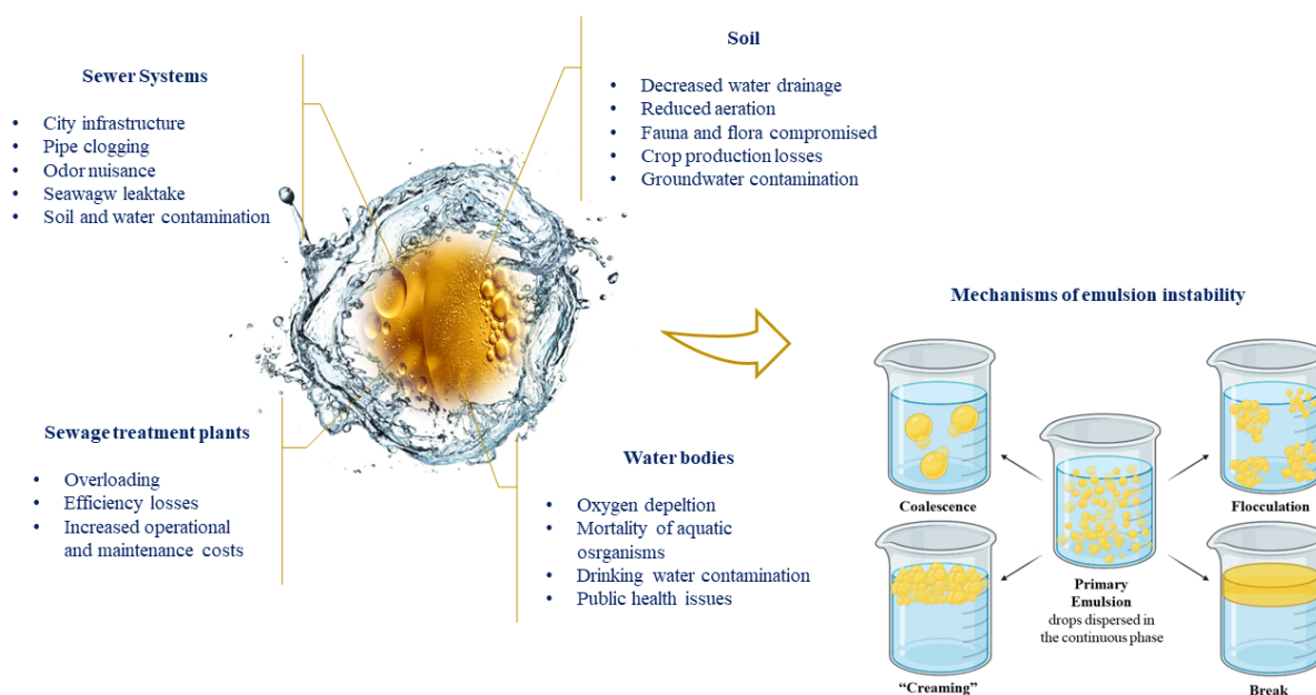
Figure 2.1. Oily wastewater incorrect disposal and representation of the physical mechanisms of emulsion instability.
